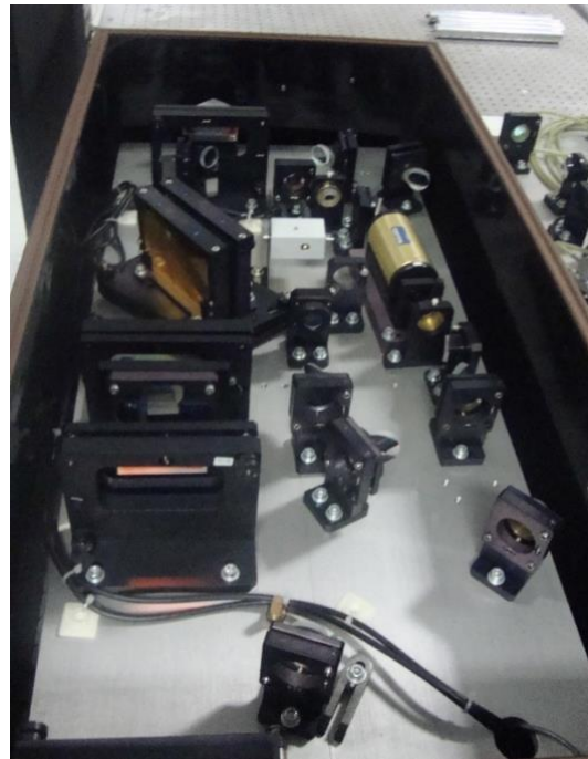
Fig. 4: Setup of in-house built 266nm 200fs high power laser source for integration in the relevant TRKR setup at the Institute of Electronic Structure and Laser (IESL) of FORTH. Top: overall picture of the assembled parts. Bottom left: the “stretcher” assembly. Bottom right: the “regenerator” assembly.
