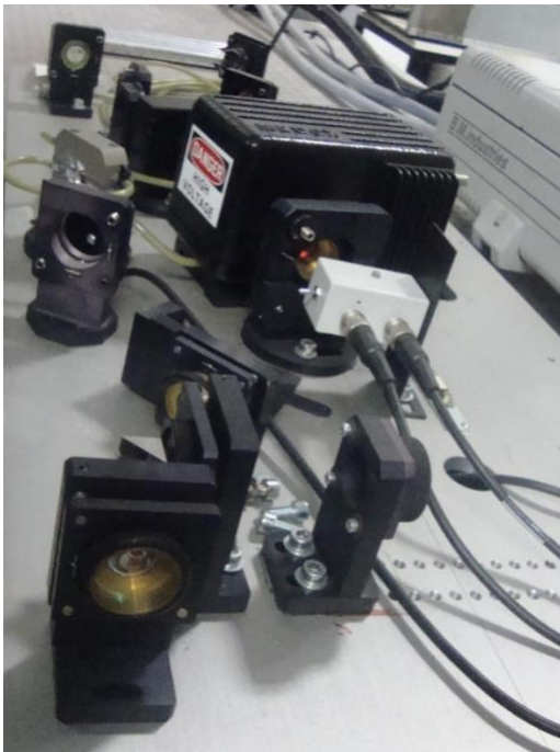
Fig. 4: Setup of in-house built 266nm 200fs high power laser source for integration in the relevant TRKR setup at the Institute of Electronic Structure and Laser (IESL) of FORTH. Top: overall picture of the assembled parts. Bottom left: the “stretcher” assembly. Bottom right: the “regenerator” assembly.
