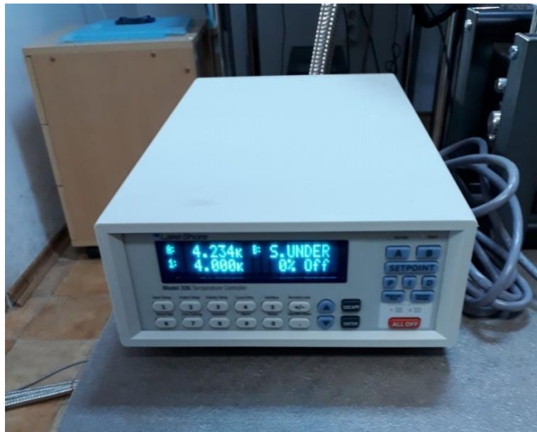
Fig. 7. Lowest temperature achieved during S-parameters tests on CS-5 kit, with the cryostat in horizontal position.
